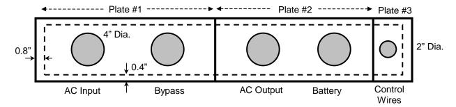
3 solid rectangles show the cable knockout plates' outline. The dashed rectangle shows the UPS opening under the plates.
